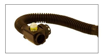
After you have taken the sensor from its bag, and it has had sufficient time to "wake-up", it can be installed into the GEM diving system. First remove the O-ring on the sensor. It is not required and will also prevent the sensor from being inserted all the way into the T-piece. Once the O-ring on the sensor has been removed, screw the sensor into position . See photo right.
