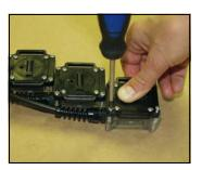
Place the back on the display case. Ensure that you have placed it correctly with the calibration port in the correct position. You will need to push it firmly down into position and must be able to hold it in place while you insert and tighten the screws. This is easiest to do by pushing down on the back, standing and using your body weight to help hold it in place.
