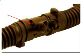
The mouthpiece is the key to the GEM diving system. The design allows gas to be eliminated from the breathing loop every time you exhale. Whether you are relaxed and not breathing hard, or you have a high work load, you will always vent the same percentage.
