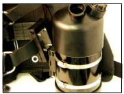
Those divers that are using a different wing/harness or BCD system, should pay attention to where they place the mounting bracket. On the system that we sell, the mount is located on the lower band. With this system, the mount is in the best position if the top band is placed as close to the top curve as possible. (where the writing is usually stamped) The bands on other systems may not be spaced the same. Our system has approximately 6.5 inches in between the bands.
