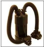
Now the remaining two loop hoses can be attached. These are the hoses with the stainless steel ballast rings. They will have the quick disconnect hose stubs on one end and the mouthpiece hose attachments on the other. These two hoses are identical. Attach the quick disconnect hose stubs to the end of each T-Piece. Ensure that the O-rings on the hose stubs have been lubricated. As per the warning above, ensure that the O-
