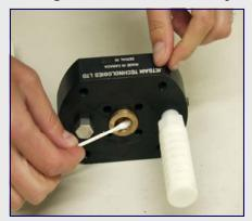
To reassemble the HP cylinder, first ensure that the cylinder is positioned so that the two screws on the HP head end are at the bottom and the single screw is at the top, as in the photo below. This is not essential, but will ensure that the fill whips end up in the proper position.
