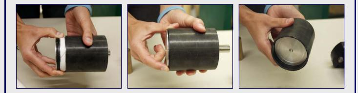
Next, push the composite tube and piston onto the JETSAM plate. The small end of the piston is inserted into the guide bushing on the HP cylinder. The piston should move freely when pushed with one finger. If it doesn't, something is binding. Once done, set aside.
