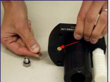
Replacing the O-rings is the only thing that can be done for these parts and even these should last many years. If you do need to replace them, cut the old ones off the valve stems and take care not to damage the O-ring grooves. Remember to lightly lubricate the new O-rings. Also, ensure that the holes that the valves go into are clean.
