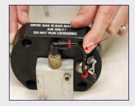
When you have the various components reinstalled on the DO NOT plate, apply a light amount of lubricant to the 041 O-ring, ensure that it is not damaged and reinstall it on the plate. Then push the plate up against the rest of the booster.
