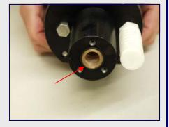
When reassembling the HP head, apply a small amount of oxygen compatible lubricant to both sides of the Reed valve, in the centre of the valves and spread it around with your fingertips. Place the Reed valve onto the head, against the O-rings and then place the valve plate on top of it. The O-rings from the valve plate should be against the Reed valve, also.
