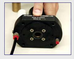
After ensuring that PV-2 is clean and that the O-ring has been lubricated, drop it back into the hole, insert the spring and then fasten the plug using a wrench. There is no need to over tighten this plug, as the O-ring creates the seal.
