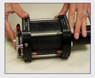
Push the HP bushing back inside the HP cylinder, with the HP seal going in first. Reinstall the 020 O-ring against the top of the cylinder after applying a light coat of lubricant.
