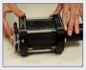
When the drive piston gets to the end of it's stroke, and has boosted the gas in the high pressure cylinder, it will run into PV-2. When this happens, PV-2 vents the signal and the Humphrey valve will stop trying to push the piston forward and vents the drive gas through the muffler. With the drive gas vented, the gas from the supply tank will start to push the piston to the bottom of the stroke again and the cycle starts over.
