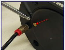
When you reassemble PV-1, you will need to push it back into the hole in the DO NOT plate as the small O-ring creates a tight fit in the hole. PV-2 will drop easily into the hole. When these plugs are correctly installed, they should protrude about 1 mm above the surface of the plates.
