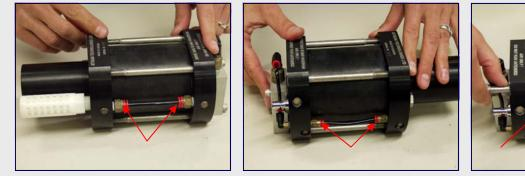
Once the DO NOT plate and the composite tube have been removed, you can see the four screws that hold the HP cylinder to the JETSAM plate. When these screws are removed the high pressure cylinder can be separated from the JETSAM plate and then you can push the HP bushing out of the HP cylinder and get at the HP seal.
