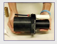
To reinstall PV-1, apply a small amount of oxygen compatible lubricant and ensure that the valve hole is clean and insert the valve. As the O-rings are a tight fit into the hole, you will need to push PV-1 into position. Once installed, the stem of the valve will protrude by about 1 mm above the surface of the plate. Tighten the plug. Do not over tighten; the O-ring is what makes the seal.
