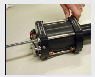
Reattach the thin hoses on either side of the booster.
