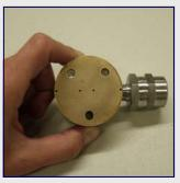
Once the HP head has been removed, the HP bushing (bronze sleeve) will need to be removed from the booster. Removing it may be tricky. First, using a piece of plastic, push the piston to the bottom of it's stroke and shake the high pressure bushing out of the front of the booster. DO NOT DROP IT! If that does not work, insert your finger into the high pressure bushing and pull it
