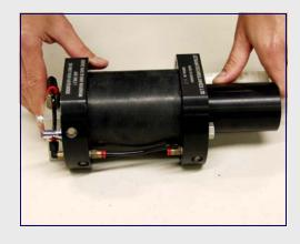
Use the 5 inch screws to secure. Remember to tighten the screws evenly. Placing the booster on a flat surface will keep the two plates in alignment.
