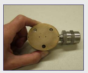
While holding the HP head together, push the 1.75 inch screws through the holes and then place against the booster and secure. Remember to tighten the screws evenly and firmly.
