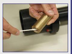
Next, insert the guide bushing into the JETSAM plate as shown in the photo below. Apply a small amount of oxygen compatible lubricant to the inside of the bushing and distribute evenly.
