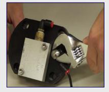
Next, install the LP inflator nipple. This also has an O-ring seal and should not be over tightened. Then, reattach the tube going to the Humphrey valve.
