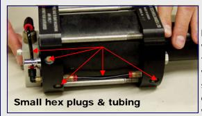
If the plugs or tube fittings aren't leaking the next possibility is that PV-1 or PV-2 are leaking. To determine which one is the problem disconnect the small tube at the "JETSAM" plate. To do this press the red ring towards the fitting and pull the tube out of the fitting at the same time. Fold the tube over to seal it and turn on the drive gas. If the booster still stutters the leak is somewhere in the "DO NOT" plate area or PV-1. If the booster
