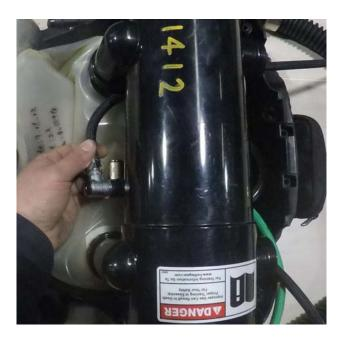
Next, connect the oxygen supply. Connect the 30" green hose (with the MAV attached) to the swivel elbow mounted to the manifold. Route this hose over the right shoulder, and attach the 36" oxygen supply hose to the manual add valve.
