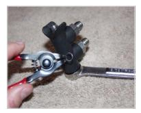
The tools required to disassemble the valve are a wrench or Allen key, small snap ring pliers and a jewellers screw-driver. First, insert the snap ring pliers into the snap ring on the button end of the valve and remove.
