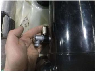
Fit the 32" black LP hose with a check valve and quick disconnect, and pass this hose over the left shoulder and under the scrubber body. Connect it as shown to the ADV; this should be where gas was supplied on the original unit. This will be the supply hose for connecting offboard diluent.
