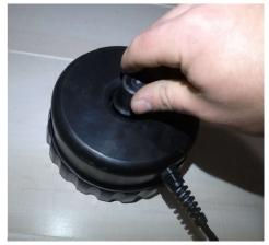
You may now secure the head to the scrubber body in the same way as the original Explorer head. Align the display cable in the correct direction before locking in the head. Do not adjust the cable position by turning the cover, as this will strain the cable and cells.
