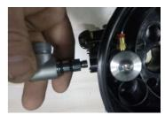
Put the retaining O-ring from the LSS module onto the oxygen injection plug, and insert it into the center of the scrubber, where the LSS module was. There should be a 113 Viton O-ring on the end of the plug, which will seal against the inside of the scrubber canister. You do not need to have the scrubber in place to install this, and the scrubber can be removed and replaced without disturbing this part, as it will seat against the head.
