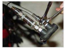
When attaching the valve to the filter and the hoses, it is very important that you use a second wrench to hold the nut next to the valve body in place. Do not allow this nut to spin as it will over-tighten and strip the plastic. This will cause the valve to leak. The valve body is not a substitute for a wrench.
