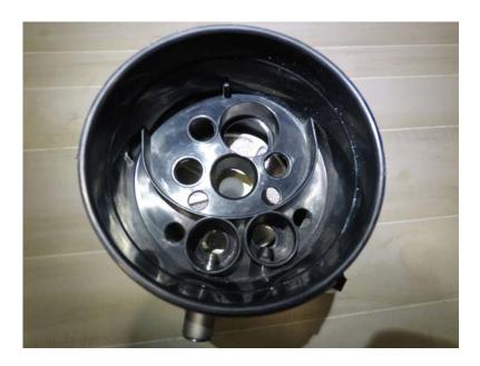
Replace the two O-rings in the swivel elbow with the Viton 013 o-rings provided in the kit. This will be where oxygen is added into the loop.
