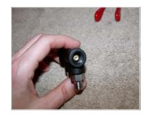
Remove the nut with either the wrench or Alan key, depending on which nut you have; pull out the spring. The spool and orifice are all that is left inside the valve.
