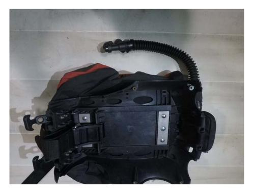
Remove the LP hose connecting the nitrox input to solenoid. Leave the fittings on the regulator, as this will serve as the ADV. The other components here, the over-pressure valve and the loop control valve, will continue to serve their functions as well.
