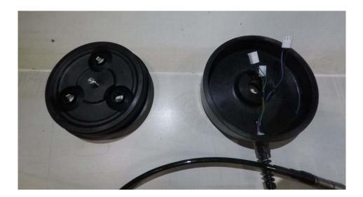
Lubricate and install the included 247 O-rings in the head. You will also need to install the O-rings you saved from the Hollis Explorer head.
