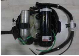
Attach the 36" black LP hose to the BOV, and attach the swivel elbow included in the kit to the other end of the hose. Run the hose over the right shoulder, and under the scrubber body. Connect the fitting to the ADV as shown.
