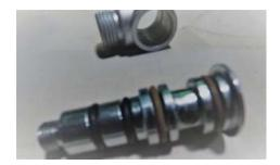
Next, put the O-ring from the solenoid onto the oxygen manifold, and push it into place where the solenoid was. This will be easier later if you have the small rubber hose already in place on the manifold. Replace the swivel fitting, and ensure that the port plug on the manifold is secure.
