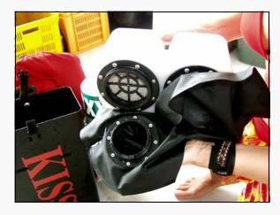
Lift the scrubber canister out of the counterlung case and remove the counterlungs. The lungs are removed by rotating them 1/4 turn counter-clockwise.
