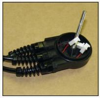
Once the wires have been secured to the connector, the other end can be attached to the display case. First, twist the wire counter clockwise 6 to 8 full revolutions. Then insert into the clear cover and tighten by hand. For the last 1/2 to full turn, use a wrench and tighten until seated. Twisting the wire prior will ensure a straight wire once you have finished reassembling the display case. Follow the directions on page 42 for reassembling the case properly.
