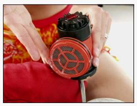
Remember to push the hose attachments on evenly and ensure that they are flush with the canister attachments and that the o-rings is not protruding.
