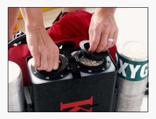
Attach the scrubber canister caps onto the top of the scrubber.
