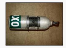
We have found that after a year or two of use, the tank mounting system can start to wear. If this happens the cylinders can pop out of the holder. First flip the mount on the cylinder. By doing this, you should get more life from the mount. Also, at some point, the lever may need to be replaced also. The lever will need to be replaced after a year or two of wear, or if it breaks.
