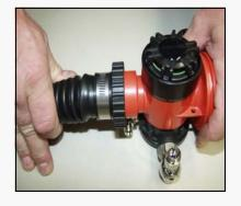
\*SERVICE: THE O-RINGS ON THE HOSE STUBS AND THE CORRESPONDING SURFACES ON THE DSV ADAPTERS AND HOSE ATTACHMENTS SHOULD BE LUBRICATED ON A REGULAR BASIS. PRIOR TO DIVING, ENSURE THAT THE HOSE ATTACHMENTS ARE PROPERLY SECURED TO THE PODS AND DSV. FAILURE TO DO SO, COULD CAUSE INJURY OR DEATH!!!
