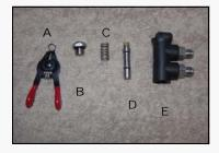
To remove the spool and orifice push in the button using a jewellers screwdriver. This will force the spool and orifice out the other end. When you have the spool removed, cut the old o-rings away with a sharp knife and replace them with new V75-OO8 o-rings which have been lubricated with an oxygen compatible lubricant such as Christolube. Do not scratch the O-ring grooves. The orifice does not need to be removed unless it is damaged or plugged.
