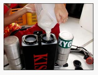
Once the canister has been replaced in the counterlung case and is secure, it is ready to be filled. Start by pouring scrubber into both sides of the canister.
