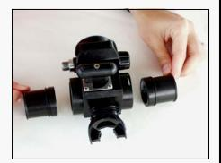
First, remove the monofilament by lifting it with a sharp dental pick and then pulling it out of the groove with a pair of pointed pliers or forceps. This will release the hose sleeve retainers.
