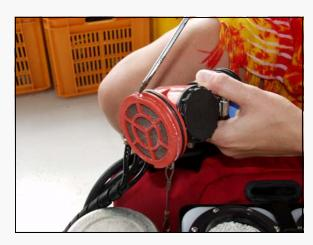
Chances are that a small amount of scrubber has collected in the edge of the hose attachments. Use a tool with a sharp end to clean out the debris. This will ensure a good seal and will make re-attachment easier.
