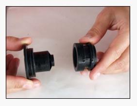
With the screws removed, turn the selector knob slightly counter-clockwise. This will cause the spool guide to pop out of position and protrude from the front of the body. Pull the knob out of the body. Once the knob has been removed, pull the spool guide and spool out of the body as well.
