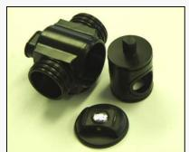
Finally, the mushroom valve carriers can be removed. From the inside the body, using either a blunt instrument or your finger, carefully push on the EDGE of the valve carrier. DO NOT PUSH ON THE CENTER AS IT WILL DAMAGE THE CARRIER.
