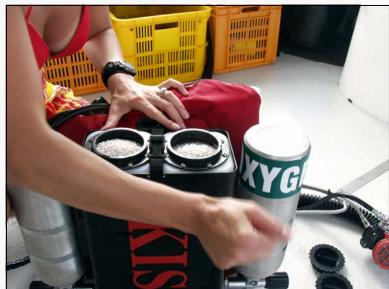
When the canister has been properly filled, the scrubber material should be level with the bottom of the black retainers.
