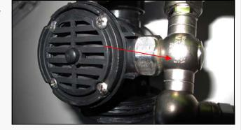
stop dropping. Also, the lungs will stop filling up all the way and the exhaust valve should stop purging. The diaphragm is simple to check. Open the cover and pull the assembly out. It should be fairly flat, and not damaged. You may need to look quite closely for small tears or holes. Sometimes holding it up to the light and gently pulling the rubber will help.
