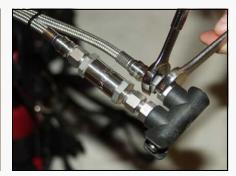
When attaching the valve to the filter and the hoses, it is very important that you use a second wrench to hold the nut next to the valve body in place. Do not allow this nut to spin as it will over-tighten and strip the plastic. This will cause the valve to leak.
