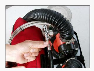
Changing the scrubber on the Sport KISS is quick and easy and takes just minutes. To start, unclip the two quick link tethers and remove the rubber LP hose which is connected to the inside of the T-connector swivel. The quick link/split ring tethers keep the pods from spinning and also hold the scrubber canister in place.
