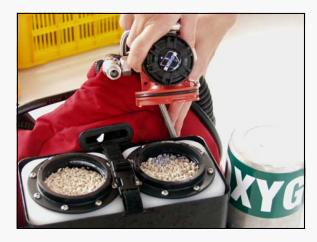
Remove the two hose attachments by rotating them 1/4 turn counter-clockwise and pulling up.
