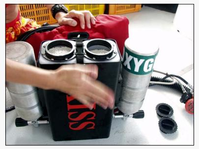
The final topping up of the container may require small amounts of scrubber being added along with slapping or shaking to settle it.
