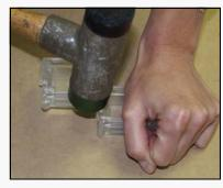
Apply lubricant to the puzzle pieces which join the displays together and then push the pieces together by hand. (ensure that you have them oriented the correct way). You should be able to push them about 1/8 to 1/4 inch together. Then, lay the cases on the table and gently tap with a rubber mallet until the edges on the back are even. Tap gently in the area where the cases join. See photo on the left.
