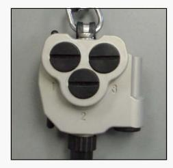
The VR Technology pendent display has 3 PPO2 readouts which read 3 individual sensors, an independent battery compartment, and 3 calibration potentiometers, one for each sensor. This is a great display for those who want a simpler system for battery changes and calibration. As the case is not opened during calibration there is less risk of flood damage. Also, the battery change is quick and simple as only one part needs to be undone. This makes any last minute battery changes simple and fast!
