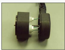
Attach the sensor assembly to the display pod, ensuring that the N70-034 O-ring on the sensor assembly is in place and lubricated. The assembly needs to be attached to the side of the pod which has a groove machined into it. Please see the photo to the right and to the bottom for groove placement. The flat edge of the sensor assembly needs to be positioned at the bottom side of the pod.
