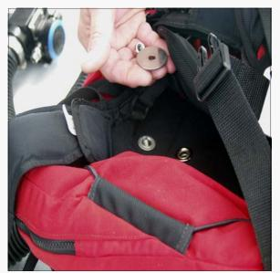
To attach the BCD lay the unit down, front side up. The BCD should be positioned so that it sits as low as possible. The higher the Sport KISS sits on the divers back, the better the work of breathing will be.
