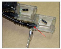
\*NOTE: Do not touch the other nut on the strain relief. This is used to attach the strain relief to the wire. Generally, a strain relief can only be used once. If you loosen it or remove it, it should be replaced. Also, it is normal for the 2 nuts to have a gap between them.
