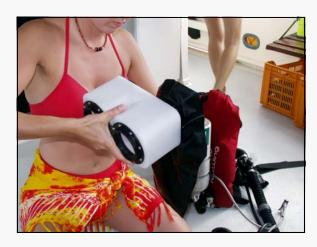
Rinse out the canister with fresh water to remove any old scrubber material. Once clean, disinfect the canister, lungs, breathing hoses and DSV if necessary. Ensure that the o-rings on the counterlungs and attachment areas of the canister are clean and free of debris and apply a small amount of lubricant. Re-attach the lungs to the scrubber canister. Remember to push them on straight and ensure that the o-ring is not pinched.
