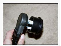
Plug the sensors into the white molex connectors. Once connected, check the displays to see if you are getting "negative gas". If you have a minus sign in front of the reading, you will need to turn the corresponding molex connector around. This will eliminate the minus sign. Unfortunately, there is no way to determine which is the correct way until you actually hook the connector up. Note that this will not effect the accuracy of the reading; it will just give you a minus sign in front of it.
